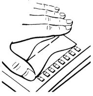
To label the fixed function keys (→ page 3), punch out the **small** preprinted labeling card. Insert the card and cover it with the plastic foil supplied (matt side up), as shown in the drawing.
