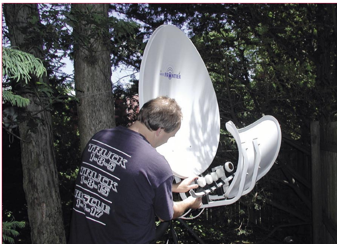
TELE-satellite editor Ron Roessel mounting LNBs on the rail of a Wavefrontier Toroidal T90 multifeed dish at TELE-satellite's Test Center in the outskirts of New York
