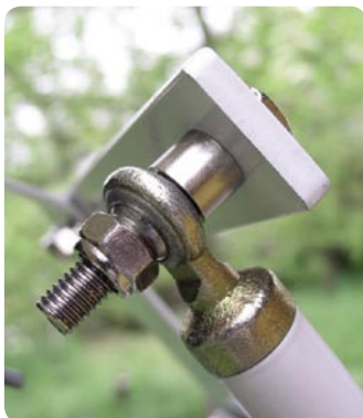
The drive joint is designed as a press bearing
