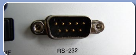
Can be found with many receivers: RS-232 plug for programming via PC
