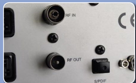
UHF connectors (left) became a rarity nowadays, instead the S/PDIF plug is more common
