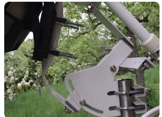
The latitude scale is used to align the dish according to the geographic latitude of the location
