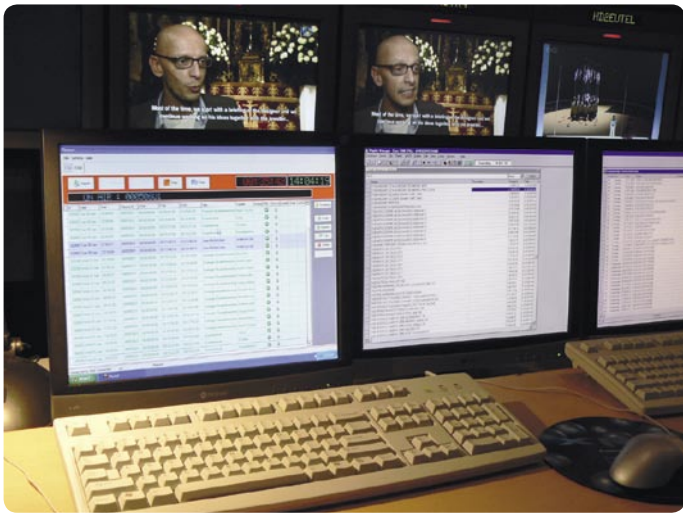
▲ The playouts runs automatically: the computers operate on one programming section after the other. The monitor to the left shows the old MPEG-2 system from EVS while the monitor to the right operates in MPEG-4 with a system from the manufacturer Grass Valley.
