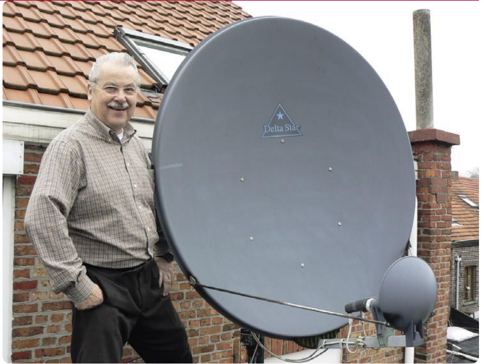
Leo Stouten on his roof next to his 1.2-meter motorized Gregorian antenna.
