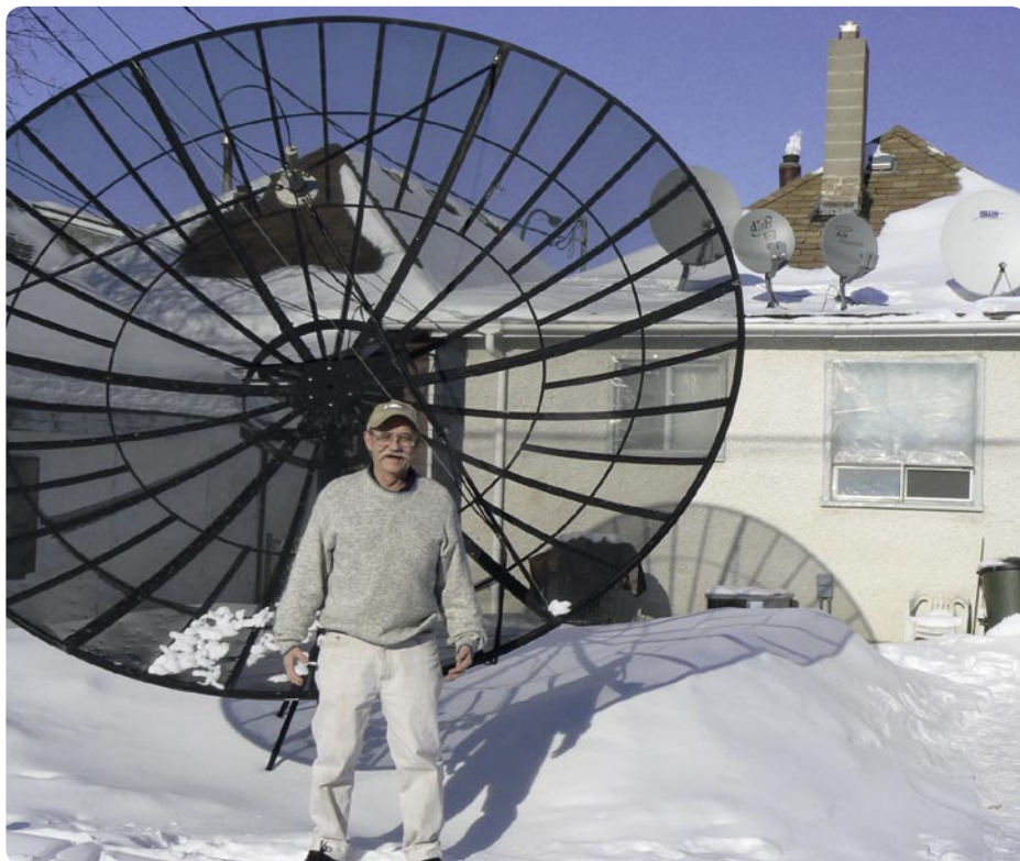
At 60 years old, Jerry is only just getting started. He is standing here in his yard in front of his 3.6-meter dish. He only just replaced the wire mesh in this dish last year. He has a C/Ku-band feed/LNB assembly installed with an actuator from the American firm VonWeise in St. Louis. His favorite satellites are SatMex 5, G3, AMC1 and Galaxy 4. The 100 cm antenna with motor he has on the roof of his house he uses to receive the satellites from
