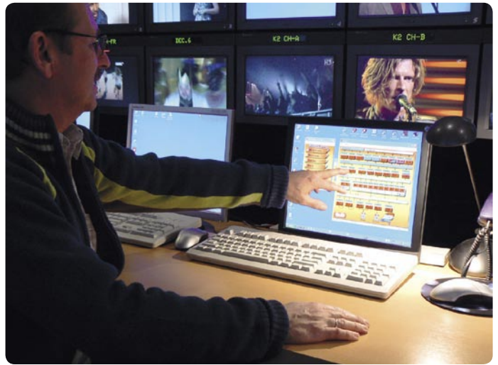
▲ Technical Director Jacques Schepers demonstrates the heart of the playout: signals can be routed to the two Astra transponders, the Eutelsat transponder or into the cable network with the click of a mouse.
