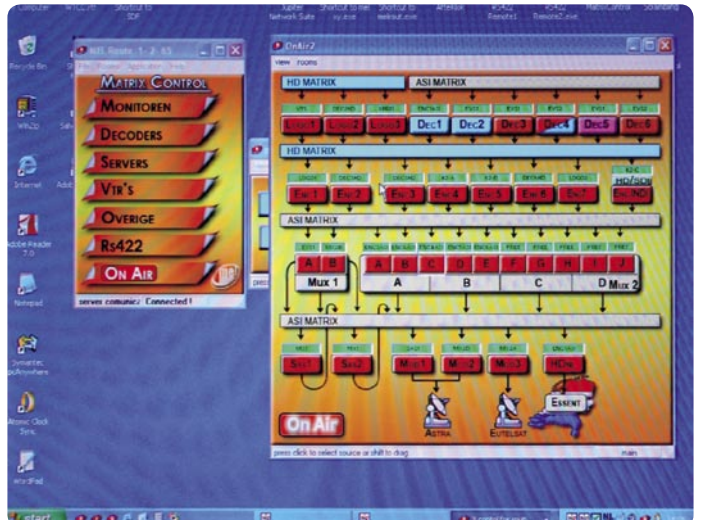
▲ Close-up of the Matrix Control with which all uplink signals can be controlled.
