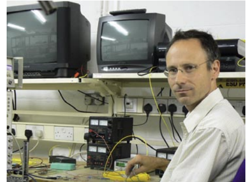
Mike checks out the prototypes. Here we see a sample product: an artificially produced satellite signal is sent over a 30-meter long fibre optic cable to a converter. He uses a test probe to determine if the original signals arrive at the analyzers within tolerance.
