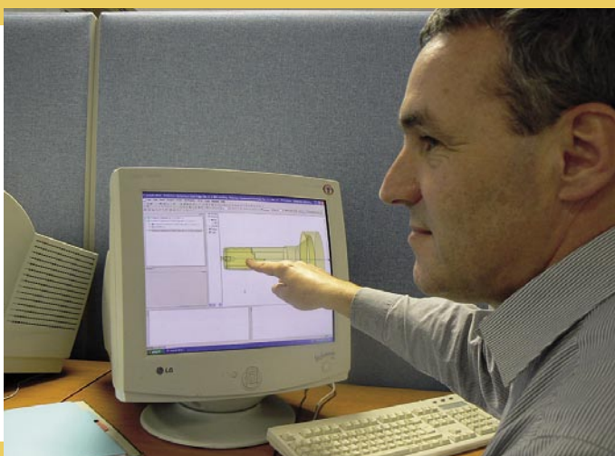
▲ How do you test the concept of your LNB? Today, this is also handled electronically. Chris Timmins demonstrates the "HF Structure Simulator" software: it simulates the behavior of an LNB and its feed. Here, Chris is in the process of optimizing the polarizer of an LNB model. He adjusts a few parameters, simulates a satellite signal and checks for any improvement.
