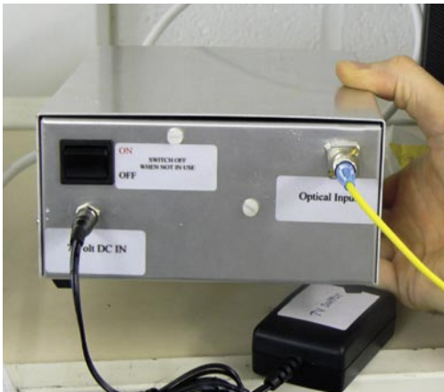
This is what the wall plate prototype looks like: the fibre optic input is on the front while the standard connection for a receiver coax cable is on the back. As you can see, the wall plate needs power. In actual use later, the wall plate will get its power from the satellite receiver's LNB input.
