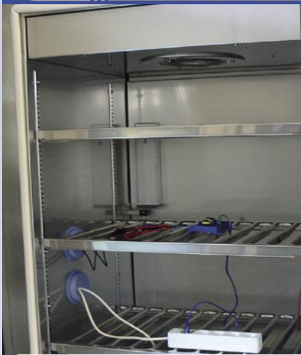
■ Completed multiswitches are also placed in this environmental chamber for testing. "Our specifications state that our devices are temperature tested from -20° C to +50° C", explains Friedrich Spaun, "but we naturally test from -30° C to +60° C to make absolutely sure."
