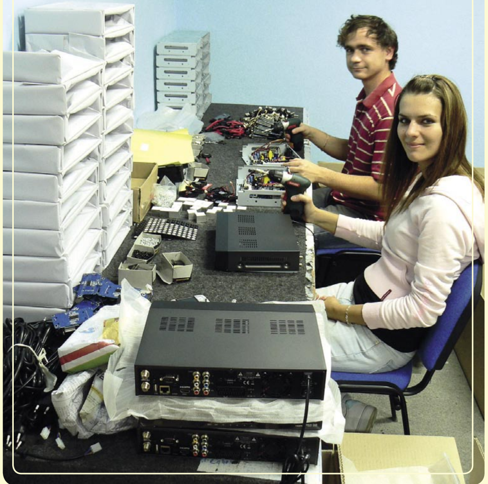
■ View of an area in the assembly shop: This is where externally sourced components are assembled by 16 employees until a finished AB-COM receiver can be individually tested for performance.
