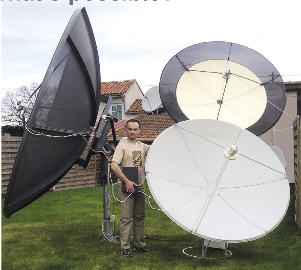
Sylvain Oscul adjusting the 1.80m prime focus dish. He can double check reception with his other 2.40m and 3.10m dishes. |
