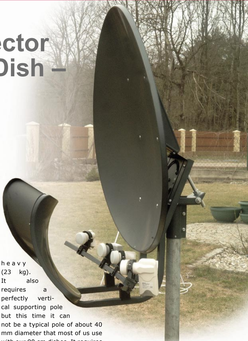
! The LNB rail of this toroidal antenna allows the mounting of up to 10 LNB for as many satellites (depending on what can be received at your location). The secondary reflector makes up for the loss in reception and allows the toroidal antenna to become equal in performance to a regular 90 cm dish |
