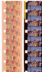
These are scans of Super 8 film. On the left is a negative and on the right is reversal.
