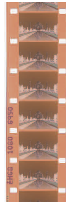
16 mm image on double-perf stock
