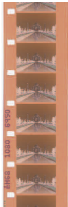
Regular 16 mm image on single-perf 16 mm stock
