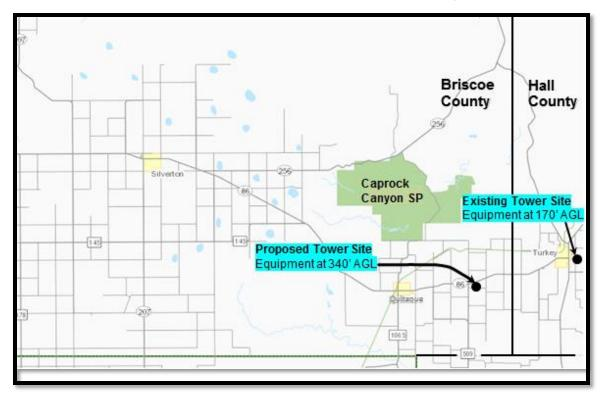
The proposed site is approximately 5.5 miles to the west of the existing site and sits 40' higher in elevation. Because it will be owned by the PRPC, the PANCOM antenna can also be raised to the top of the tower. The net gain in antenna elevation will be 170'.
