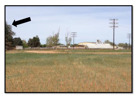
View to the northwest of the mark set for the tower location. The arrow points to the end of the windbreak that will have to be trimmed to allow clearance for the tower's northwest guywire. It's estimated that 5-8 trees be removed from this area to allow a free path for the line. The entire field was recently planted by the ISD with oat grass to keep the soil in place and blowing dust in check.
