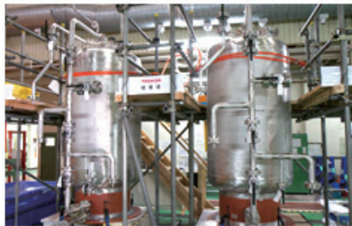
Adsorption tower of Multiple Radio-nuclides Removal System (MRRS) in the environs of Toshiba's Keihin Product Operations
