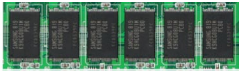
Solid State Drives use high-performance Flash Memory and have no moving parts
