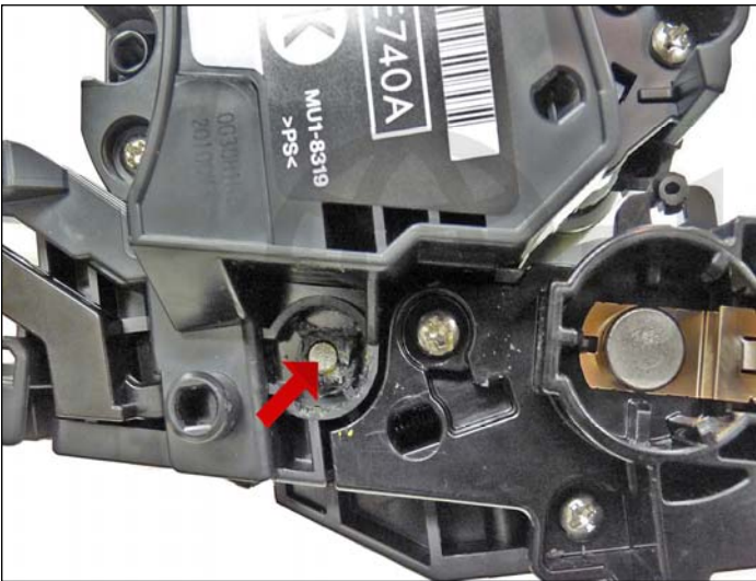
46. Install the two pins, with the large pin to the label or gear side of the cartridge.
