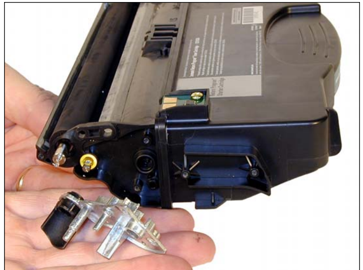
11. Remove the three screws and gear alignment plate.
