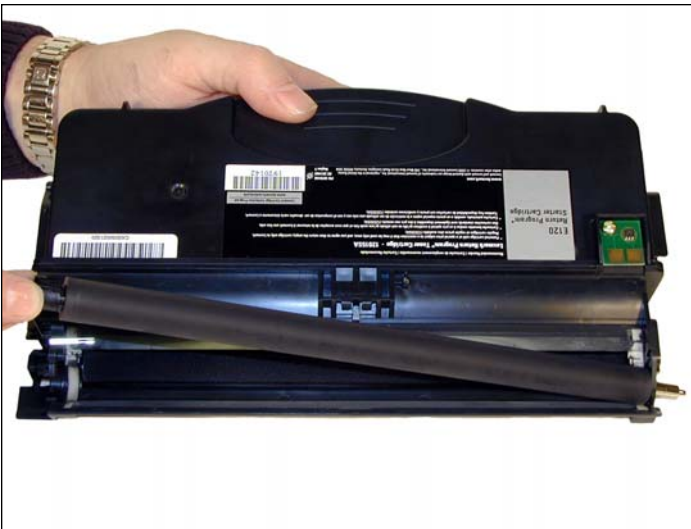
14. Lift the developer roller out of the cartridge. The bushing will come off with the roller.
