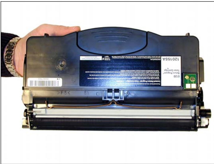
22. Install the doctor blade spring.
