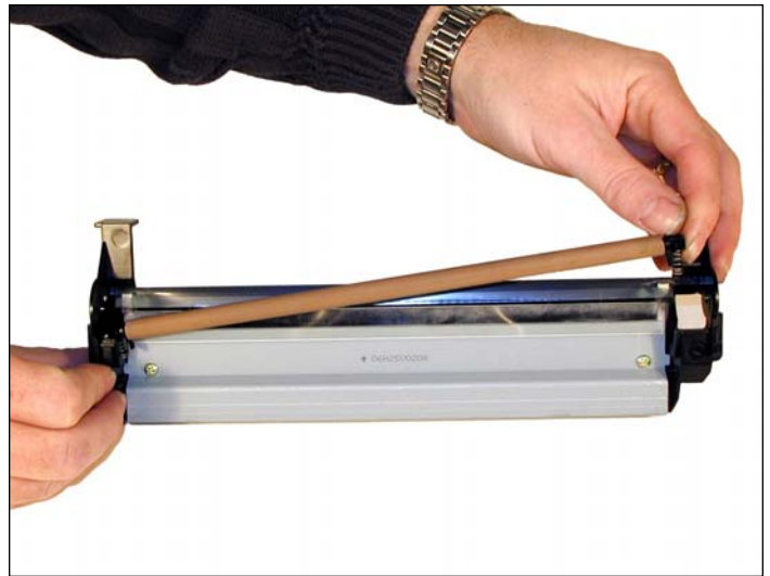
31. From the right (gear) side, remove the PCR assembly (the spring loaded holder may come with it).
