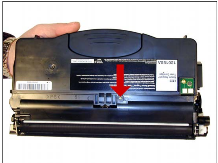
23. Install the developer roller cover and screw.
