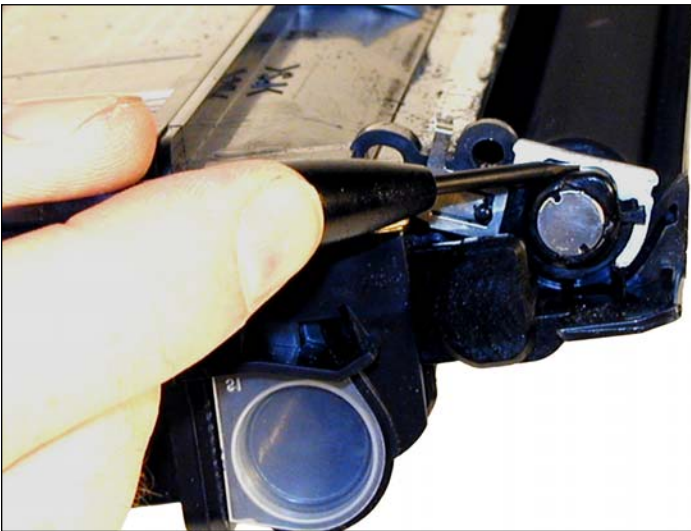
12. With a small flat head jeweler's screwdriver, pry off the metal lock from the developer roller bushing.
