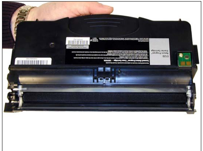
15. Clean out any remaining toner from the hopper. Make sure the developer roller retaining blade does not get damaged!
