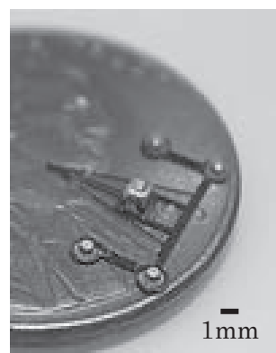
Fig.1 Micro-robot made of Si.
