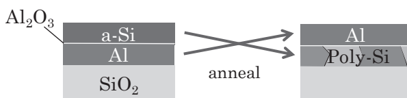
Fig. 1 Growth mechanism of AIC.
