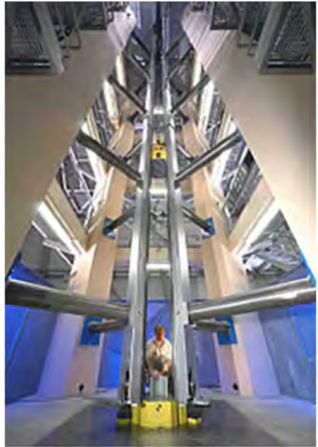
Crash tower (image courtesy of ONERA).
