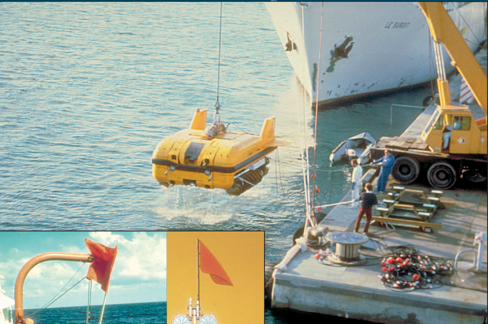
Fig.65. Photograph of the remote free-sampling device developed by Ifremer to collect polymetallic nodules © Ifremer
