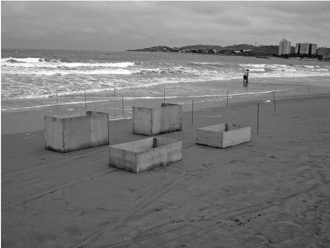
Picture 2.2.1 – Sampling protocol (beach of Playas). Wooden boxes are in place to hold the upcoming swash. In total, 8 boxes were used (only 4 shown) so 2x4 levels could be secured at the start of a sampling run (see text).
