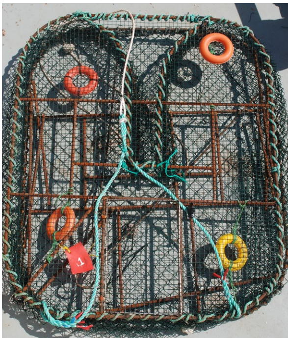
Figure 7.9 A large steel frame fish trap prototype tested on Nazareth Banks, Mauritius in 2010 (184 x 153 x 80 cm; 50 kg) (Krakstad et al. , 2010).
