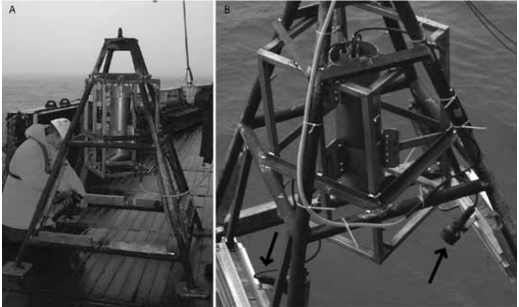
Figure 1. Underwater camcorder mounted on lander frame. A. Setup on deck. B. Detail of deep-sea camera housing, cables and spotlights (arrows).
