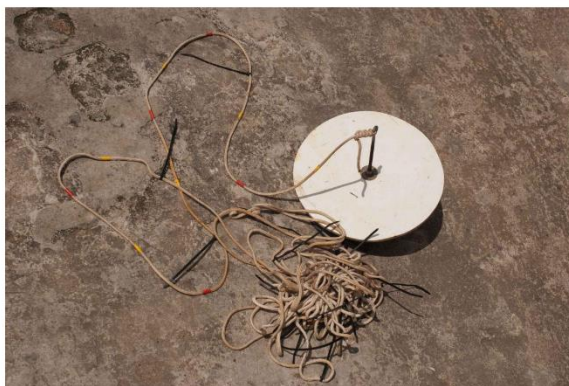
Secchi disk with markings each 0,2 m (red-yellow) and 1m (black) interval
