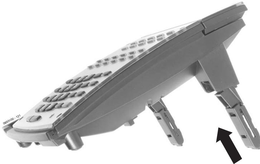
Figure 4-82: SETTING THE LEG POSITION - POSITION 3
