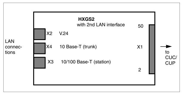
Figure 2-2 HXGS2 interfaces with 2nd LAN (S30810-Q2939-X000/X100)
