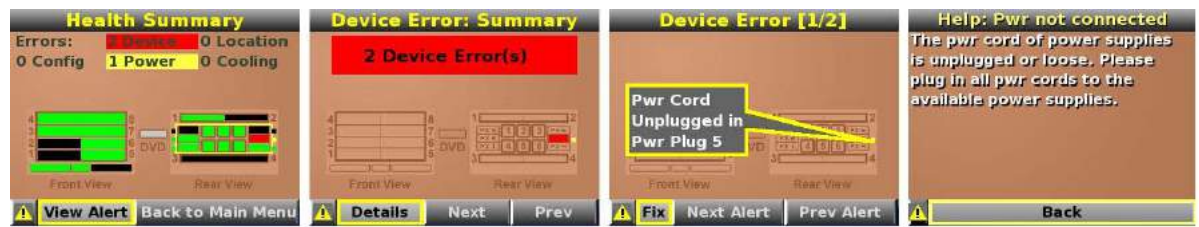
Figure 5. BladeSystem c-Class Insight Display diagnostic screens indicating an error and suggested corrective action
