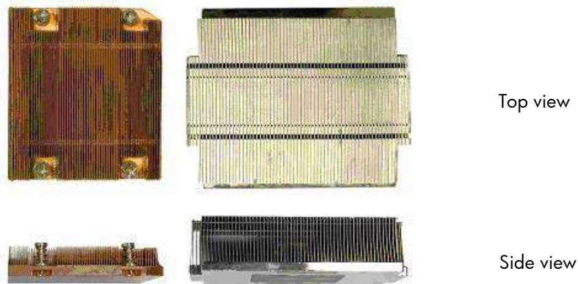
Figure 18. Processor heat sink using fully ducted design (left) and a traditional heat sink in a 1U rack-mount server (right)
