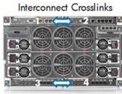
Figure 14. HP BladeSystem c3000 interconnect bay crosslinks indicated by the arrows
