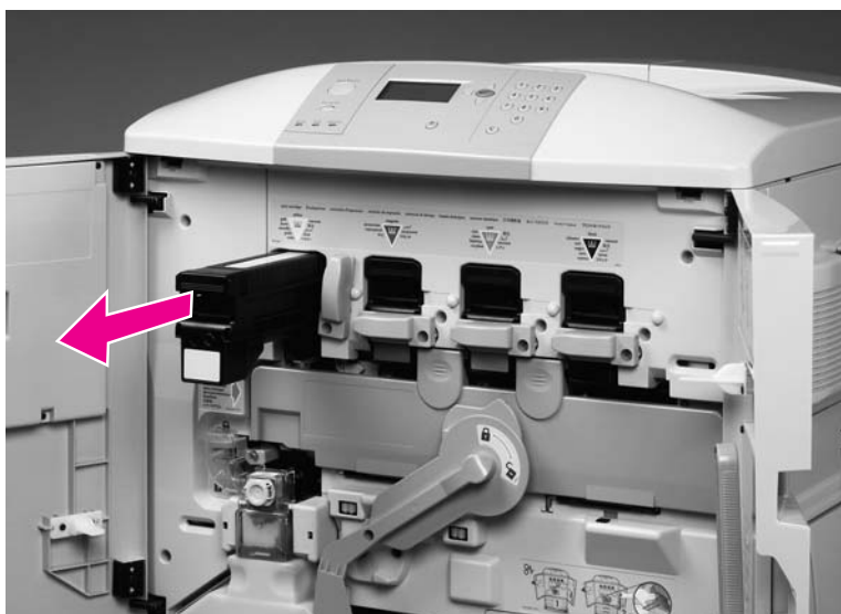
Figure 76. Remove the toner cartridge
