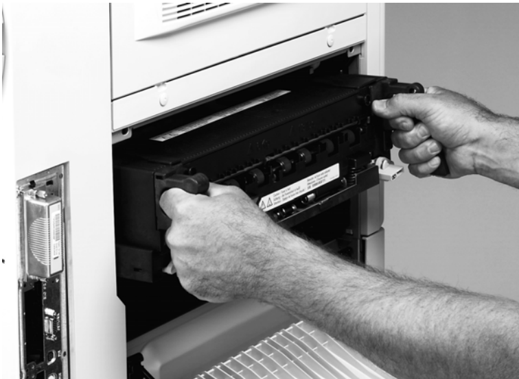
Figure 162. Remove the fuser
