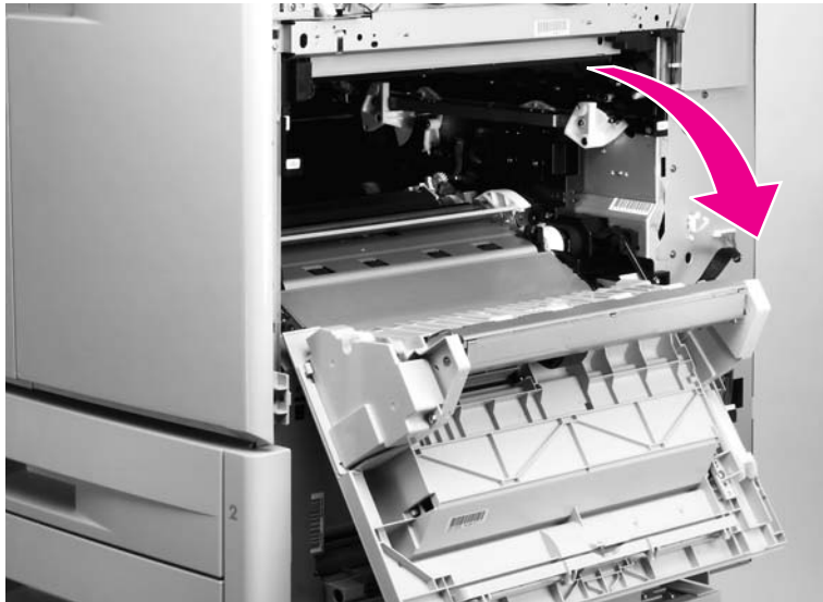
Figure 107. Open the ITB door
