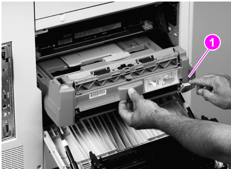
Figure 160. Remove the duplexer
