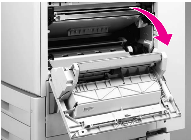
Figure 164. Open the ITB door
