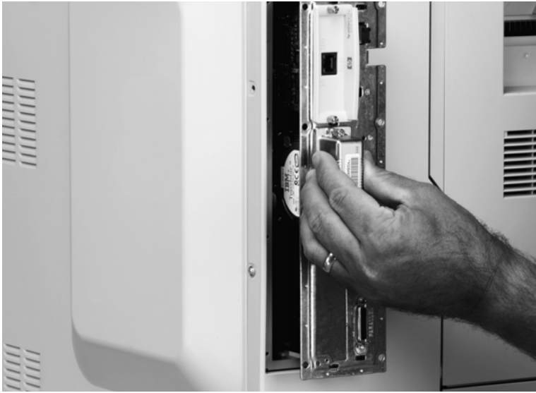
Figure 234. Remove the formatter PCB
