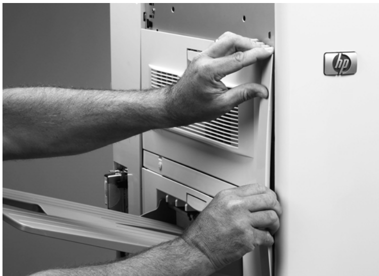
Figure 145. Remove the left side front cover
