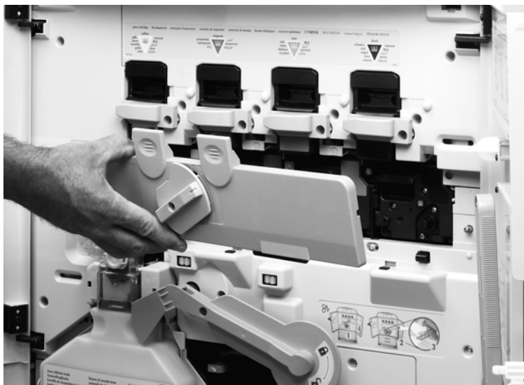
Figure 121. Remove the process cartridge door
