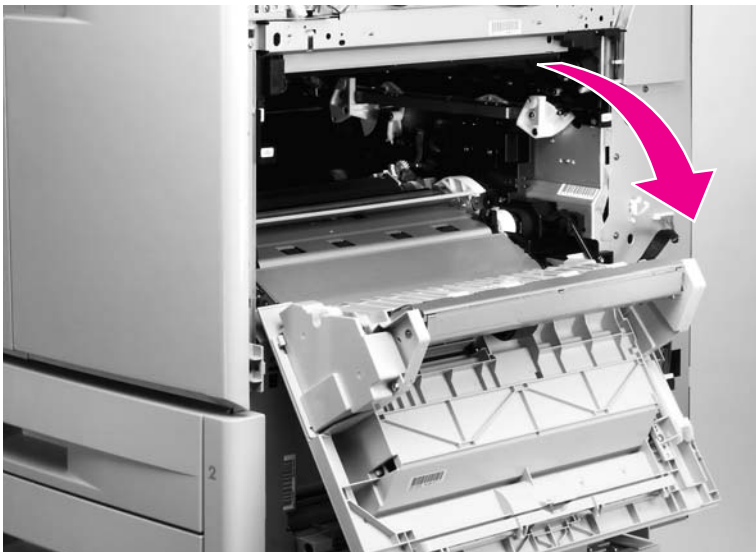
Figure 186. Open the ITB door
