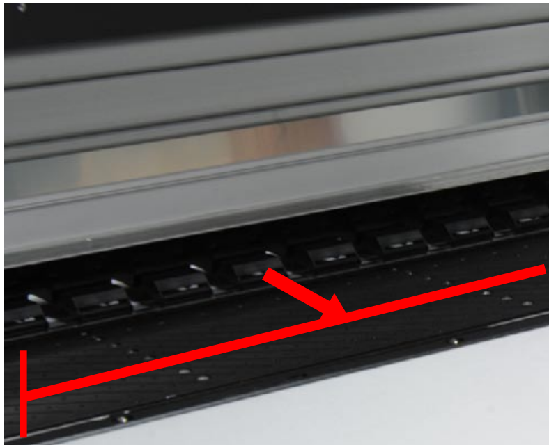
The vacuum system draws the media to the platen.
