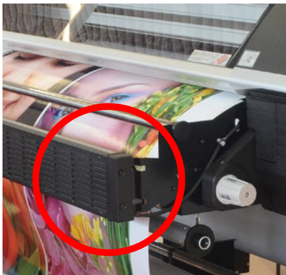
At the front the printer also has a Media dryer fan that helps drying ink after printing.
