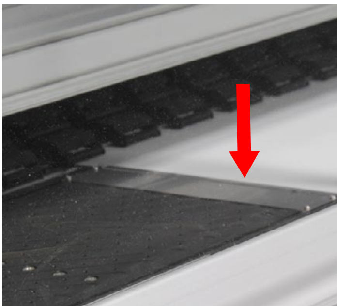
The media edge guards are located at both sides of the media, you can move each one individually.
