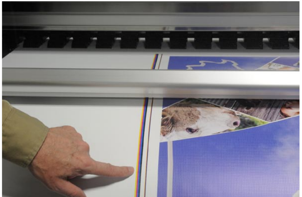
To keep all printheads fresh and avoid them to dry out when not be used you can print a band of printable colors along the edge.
