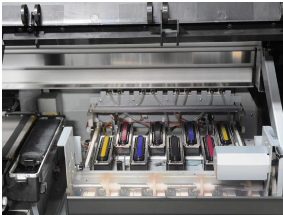
At the right side is located the capping station, that has the capping area, which prevents the nozzle of the printheads from drying.
