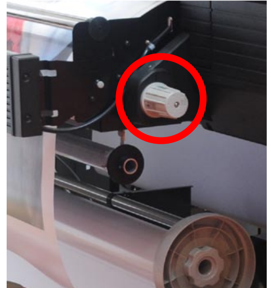
At the front and behind the printer there is a pressure control knob that adjusts the pinch rollers at four positions: High, Normal, Low and Open
