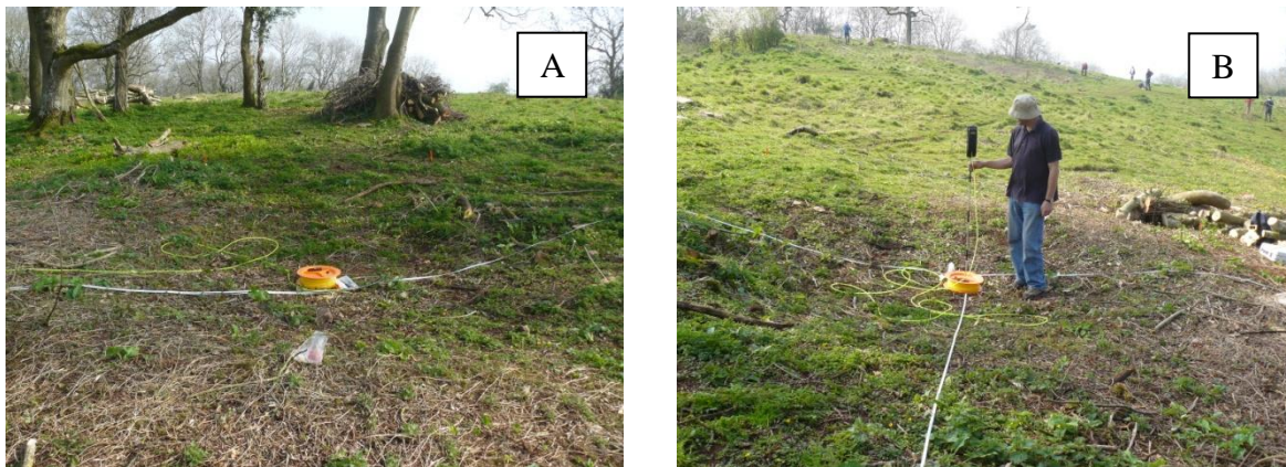
Figure 10. A, The electronic hydrostatic level is shown in the centre of the feature. B, using the level to measure heights above and below the zero point.
