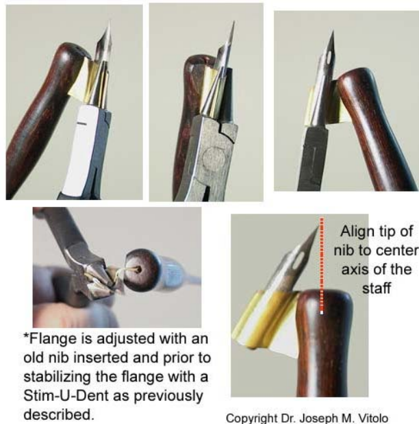
Figure 4. Adjusting the flange before fixation
