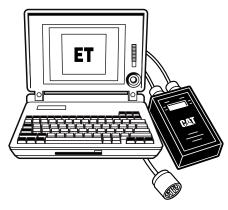
**Cat Electronic Technician (ET).** Is a software program which allows the service technician to find and identify a problem on a machine and to analyze how to fix it quickly. Cat ET provides the capability to access the electronic control modules from a personal computer.
