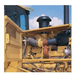
**Left Side Service Access.** Provides convenient entry to the engine oil filter, grease points, air filter, power train oil dipstick, coolant sight gauge, power train oil fill, power train oil filler and high speed engine oil fill.
