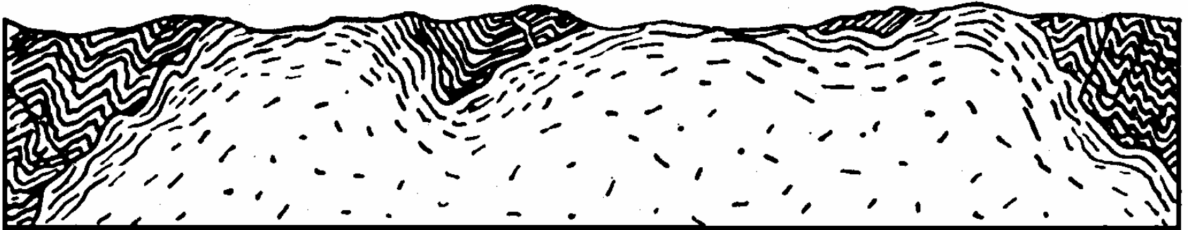
Figure 4-28. Marginal foliations developed within a pluton as a result of differential motion across the contact. From Lahee (1961), Field Geology . © McGraw Hill. New York.
