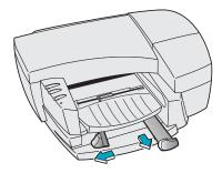
3 Place a stack (up to 5/8 in. or 16 mm thick) of paper, transparencies, or envelopes print side down in the IN tray with the right side of the stack against the right side of the tray, and push in the stack until it stops.
