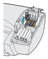
4 Grasp the top of the used printhead by its handle, and pull it up and out of its socket.
