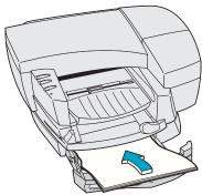
4 Place a stack of paper, transparencies, or envelopes print side down in the tray with the right side of the stack against the right side of the tray. The accessory paper tray will hold up to 250 sheets of paper (a stack up to 1 in. or 26 mm thick).
