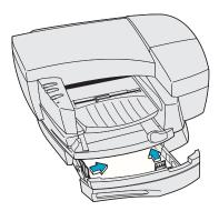
6 Close the cassette drawer. If the drawer has been removed from the tray, rest the drawer on the same level surface as the tray, align the drawer to its opening, then push the drawer into the tray.
