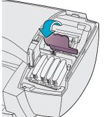
b) Push and lift the latch toward the back of the printer so the printheads are completely revealed. The latch should rest on the back of the printer.
