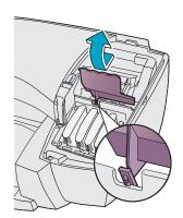
8 Replace the printhead access cover. Align the back first, then lower the rest of the cover down. Snap the cover in place and close the ink cartridge door.
