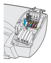
6 Holding the printhead by its handle, match the printhead label color to the socket label color. The ink connector pin should be positioned toward the front of the printer.
