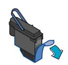
5 Remove the new HP No. [10] Printhead from its package and hold it by its colored handle. Being careful not to touch the gold-colored metallic strip on the printhead, gently remove the transparent protective tape covering the electrical contacts and ink nozzles.
