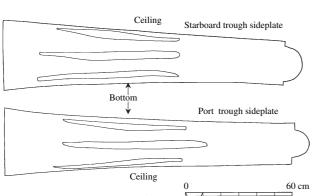
Fig. 6. The interior of the sideplates showing the dimensional variations in the plates and fin channels. (Drawing by A. Schreur and the author)
