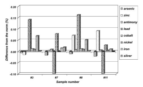
Fig. 11. Difference from the 'norm', analysis of trace elements in samples from repaired areas on the ram.
