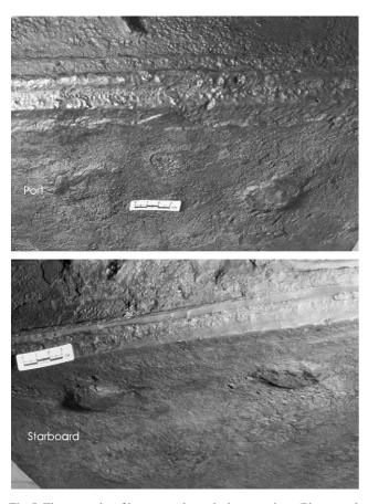
Fig. 7. The two pairs of bronze studs on the bottom plate. (Photograph by the author)
