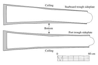
Fig. 8. Cowl ceiling and bottom plate wall thickness. The cross sections show the cowl ceilings and bottom plate wall thickness at their junction with the trough sideplates. (Drawing by A. Schreur and the author)
