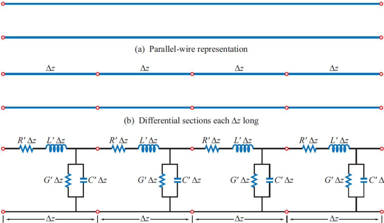
(c) Each section is represented by an equivalent circuit
