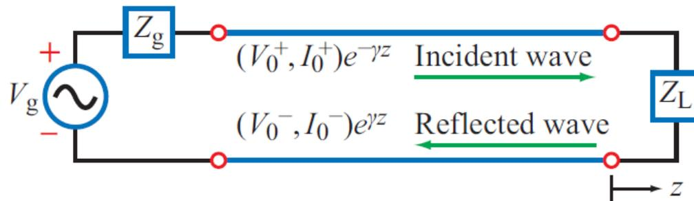
*The presence of two waves on the line propagating in opposite directions produces a standing wave.*
