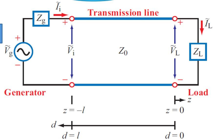
Remember: Standing wave is created due to **interference** between the traveling waves (incident & reflected)
