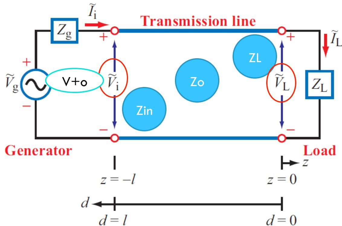
What is the voltage/current magnitude at different points on the line in the presence of load??
