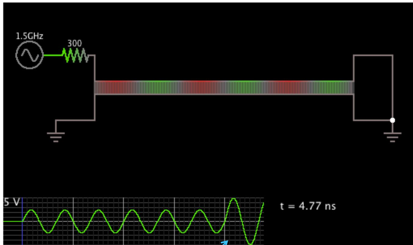
Due to standing wave the received wave at the load is now different
