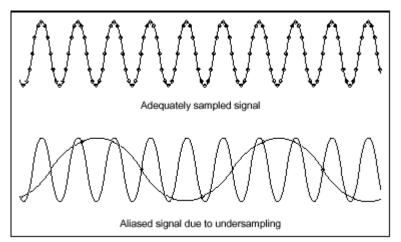
Figure 3. Adequate and Inadequate Signal Sampling
