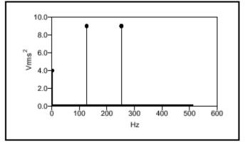
Figure 2. Single-Sided Power Spectrum of Signal in Figure 1
