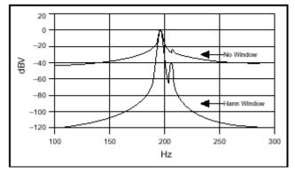
Figure 9. Spectral Leakage Obscuring Adjacent Frequency Components
