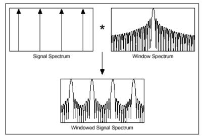
Figure 10. Frequency Characteristics of a Windowed Spectrum
