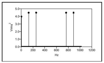
Figure 1. Two-Sided Power Spectrum of Signal
