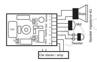
The drawing shows the connection of a 3-way system to one channel. The other channel is connected in the same way. The tweeter and mid levels are adjustable in two steps as described below:
