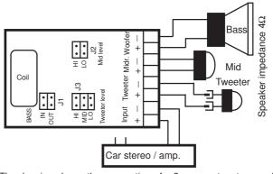
The drawing shows the connection of a 3-way system to one channel. The other channel is connected in the same way. The tweeter level is adjustable in three steps, the MID level in two steps:
