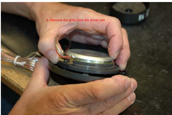
3. Remove the grille from the driver unit like this.
