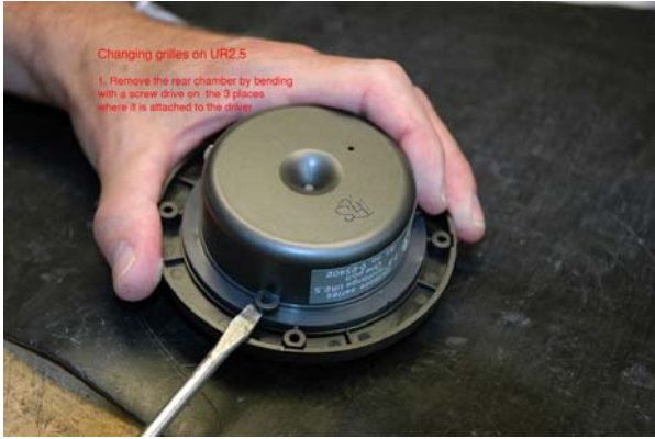
1. Remove the rear chamber by bending with a screwdriver on the three spots where it is attached to the driver. Be careful!
