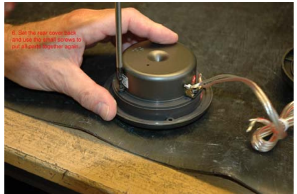
6. Reinstall the rear chamber and use the screws to put all parts together again.
