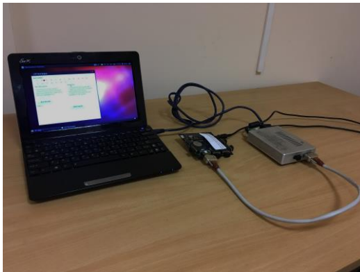
Fig. 8. SUAI Software-to-Hardware tester for STP-ISS connected with DUT via Ethernet-SpaceWire Bridge
