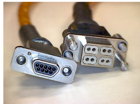
Fig. 8. 9 way micro-D connector (left) and MicroMach SpW connector (right)
