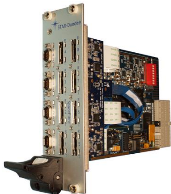
Figure 3. PXI Board configured as SpaceFibre Router. The front panel has 8 SpFi ports and 4 SpW ports
