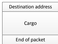
Fig. 12. Format of SpaceWire packet
