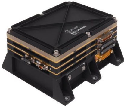
PIU: RS-422 to SpaceWire bridge
