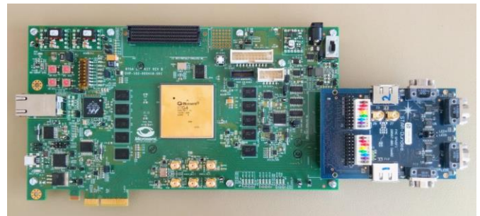
Figure 3. Microsemi RTG4 development board used to test the SpaceFibre interface
