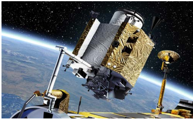
Fig. 4 - e-Deorbit concept for ENVISAT capture ([19])
