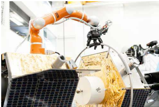
Fig. 5 – Spacecraft gripping demonstration, source DLR [23]
