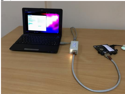
Fig. 7. SUAI Software-to-Hardware tester for STP-ISS connected with DUT via SpaceWire Brick Mk2
