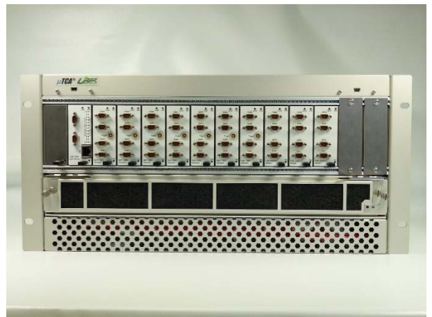
Fig.6. SpW backplane 12slots
