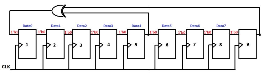
• For 16/32bit data width, same PRBS9 will be shifted 16/32 times to form Data[15:0]/Data[31:0] output respectively
