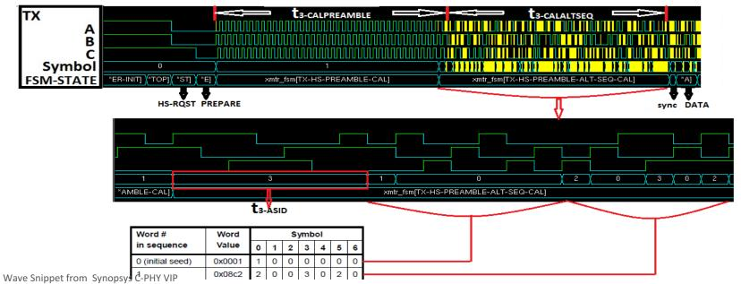
t<sub>3-CALALTSEQ</sub> For transmitter it ranges from 7UI to 14336 UI; receiver should specify required minimum; max for receiver is 14336UI
