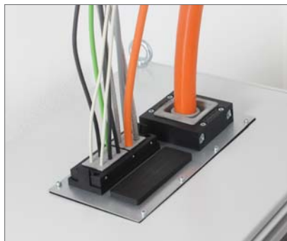
Routing of several cables with and without connectors through a closed enclosure roof via module plates. Cut-out size 314 x 144 mm.
