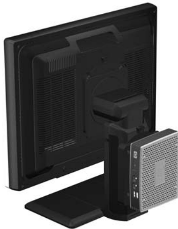
Figure 2-6 Thin client mounted on back of monitor stand
