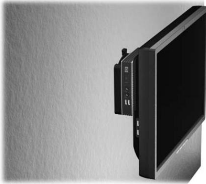
Figure 2-5 Thin client mounted with flat panel on wall
