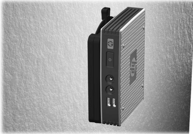
Figure 2-7 Thin client mounted on wall
