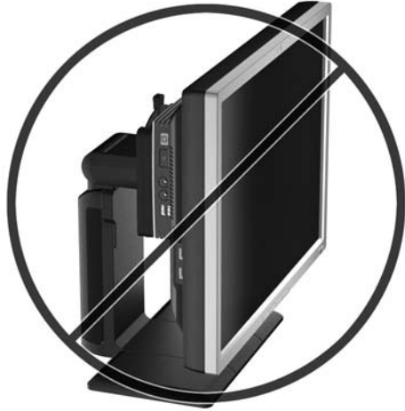
Figure 2-9 Unsupported mounting position—thin client between stand and monitor
