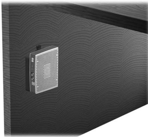
Figure 2-8 Thin client mounted under desk
