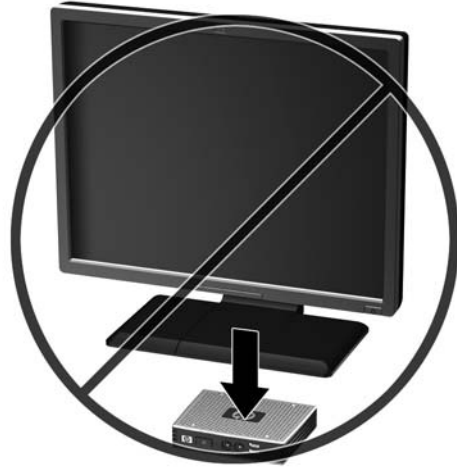
Figure 3-4 Do not place a monitor on the thin client
