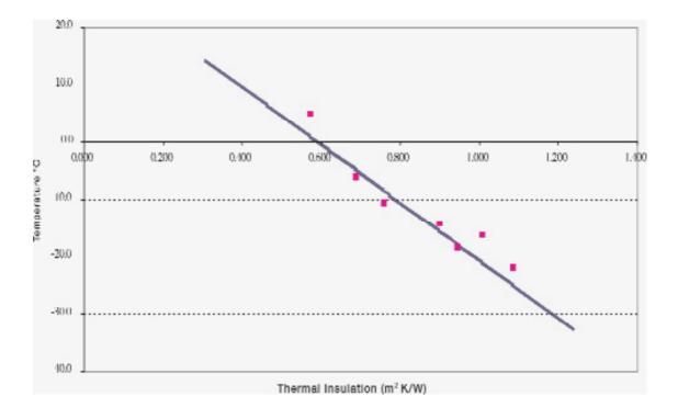
The figure shows a comparison between human evaluations of 7 sleeping bags (squares) with known thermal insulation, and predicted comfort values (solid line) based on the comfort model.
