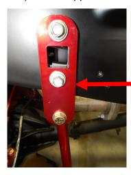
Passenger side sway bar end link mount shown using factory bolts
