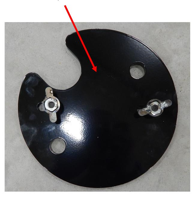
6. Locate the passenger side upper air bag mount (Part # 69049). It fastens to the bottom of the frame with the  $3/8 \times 1$ " counter sunk bolts, factory hitch with the  $5/8 \times 2$ " bolts and side of the frame with two  $5/8 \times 4$ " bolts. Torque the 3/8" bolts to 45 ft./lbs. and the 5/8" bolts to 155 ft./lbs.
