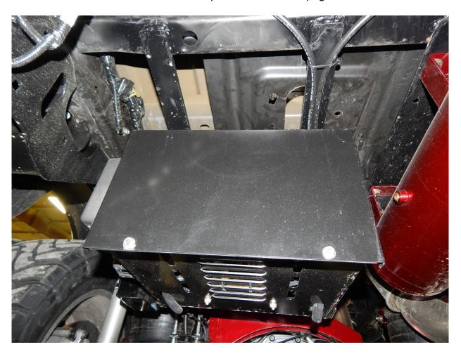
The air compressor box for the mechanical system will also mount where the spare tire normally is. The mechanical system normally only uses one tank, so you can mount it right beside the box.
