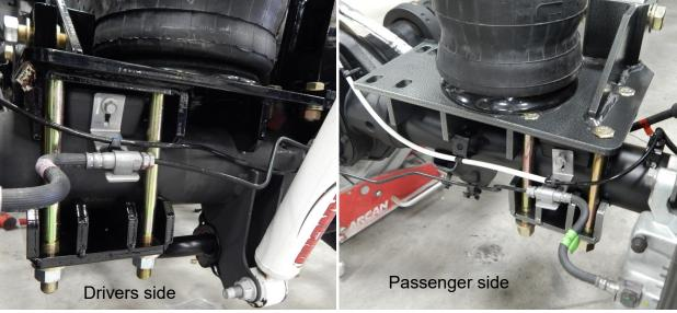
5. Locate the driver side upper air bag mount (Part # 69048). It fastens to the bottom of the frame with the  $3/8 \times 1$ " counter sunk bolts and nut tabs. Torque the 3/8" bolts into the bottom of the frame to 45 ft./lbs.
