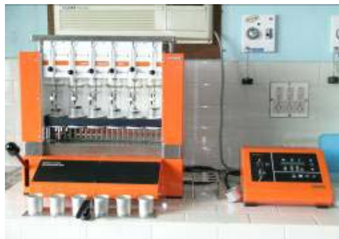
8. SOXTEC SYSTEM 2043 FOSS Analytical AS, France for solvent extraction of oleoresin
