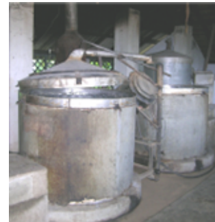
6. Field distillation unit
