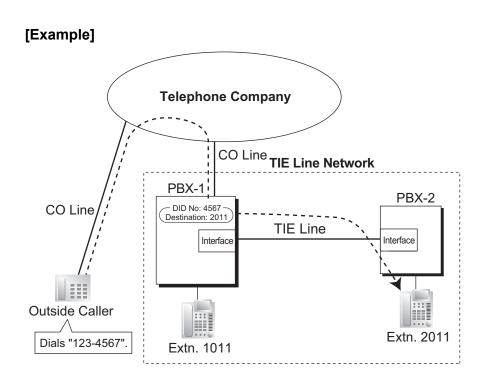
An outside caller dials "123-4567". The call is sent to extension "2011" of PBX-2 through the TIE line according to the assignment of the DID or DIL call destination of PBX-1. ( $\rightarrow$  4.1.6 DID (Direct Inward Dialing))
