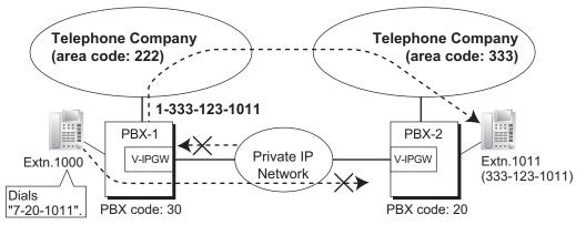
The leading numbers of extensions accessed through the VoIP network are added as entries to the Quick Dialing table, in addition to being registered as Other PBX Extension Numbers, as shown below:
