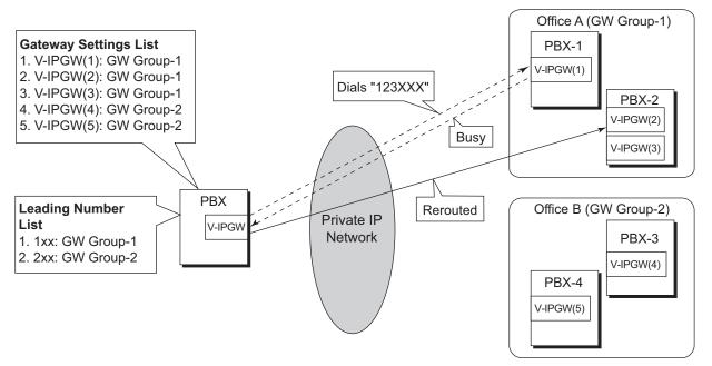
When "123XXX" is dialed, the call is routed to GW Group-1. However the lowest-numbered device (V-IPGW(1)) is busy or not available, so the call is rerouted to V-IPGW(2).
