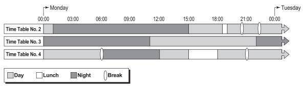
Note that time modes can be arranged as they are needed (for example, night mode can occur in the morning and afternoon, if necessary) and not all time modes need to be used in a tenant's time schedule. Also note that Tenant 4's Break 1 is followed by the night mode because no end time is programmed for the break.
