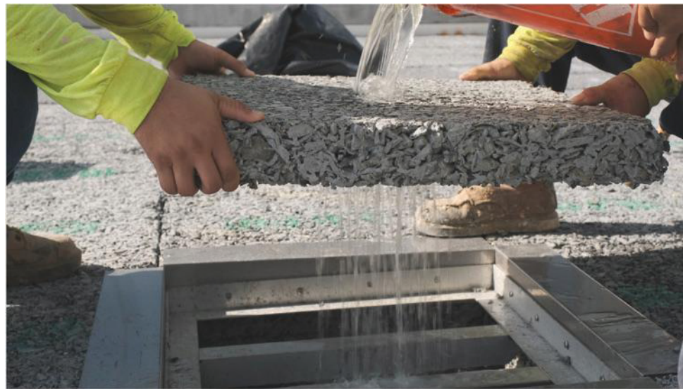
Echo Flow recycled rubber concrete blocks provide superior drainage on the rooftop terrace.
