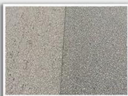
FIGURE 2 East Lansing, Michigan (L) Superpave 5E Mix (R) Same recipe utilizing SmartMIX
