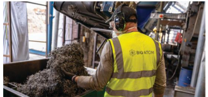
UK tire processor Big Atom extracts two grades of tire wire from its end-of-life tire processing operation
