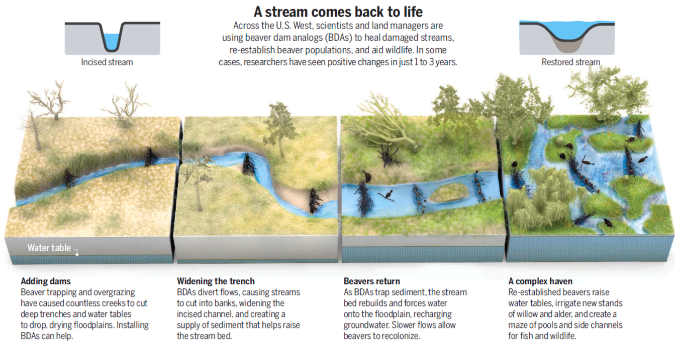
Fig. 2. Illustration of the process of encouraging beaver dam activity with beaver dam analogs (BDAs) and how this can lead to (on right) self-sustaining Stage Zero conditions (anastomosing or multi-threaded channels around island complexes). (Source: Goldfarb, 2018b).
