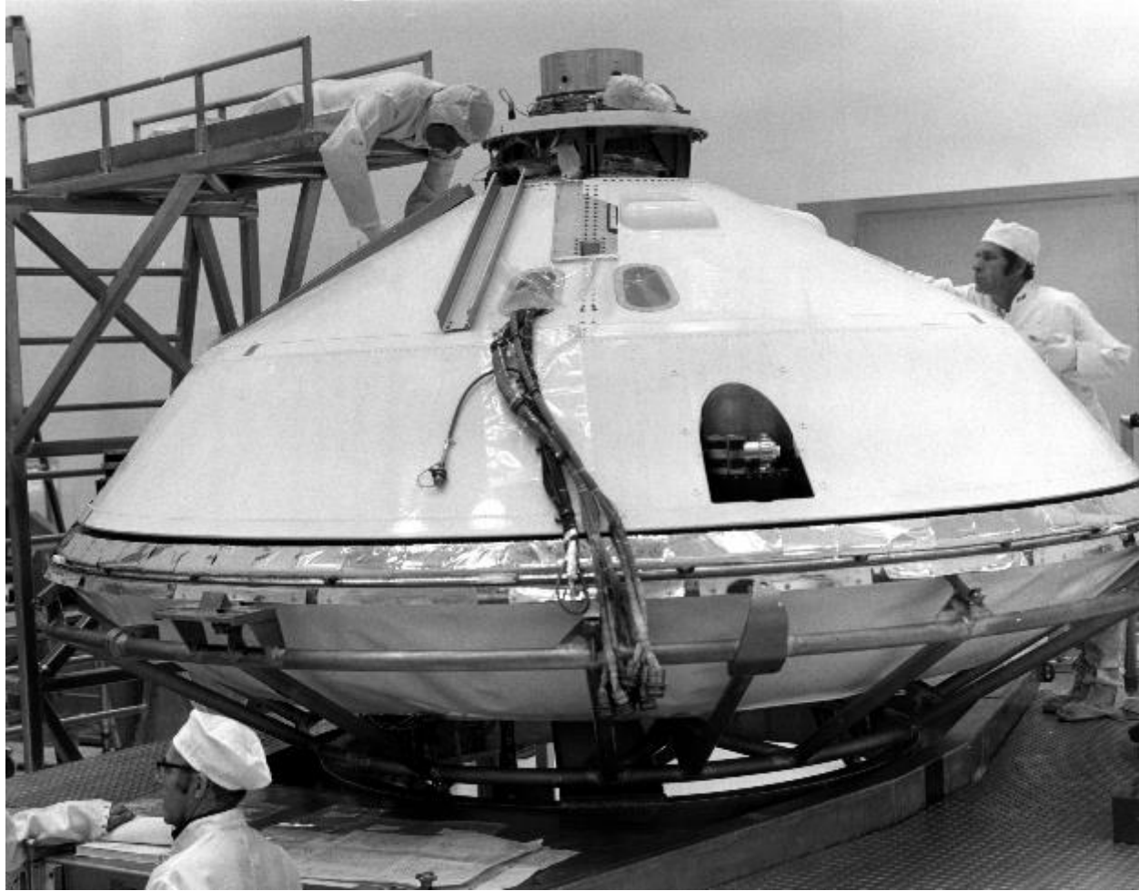
FIGURE 2.4 One of the Viking landers sealed in its protective bioshell to prevent recontamination after dry baking in a specially constructed oven at 111.7°C for more than 30 hours. SOURCE: Courtesy of NASA. https://www.nasa.gov/centers/kennedy/about/history/50thgallery/1975-01-07.html .
