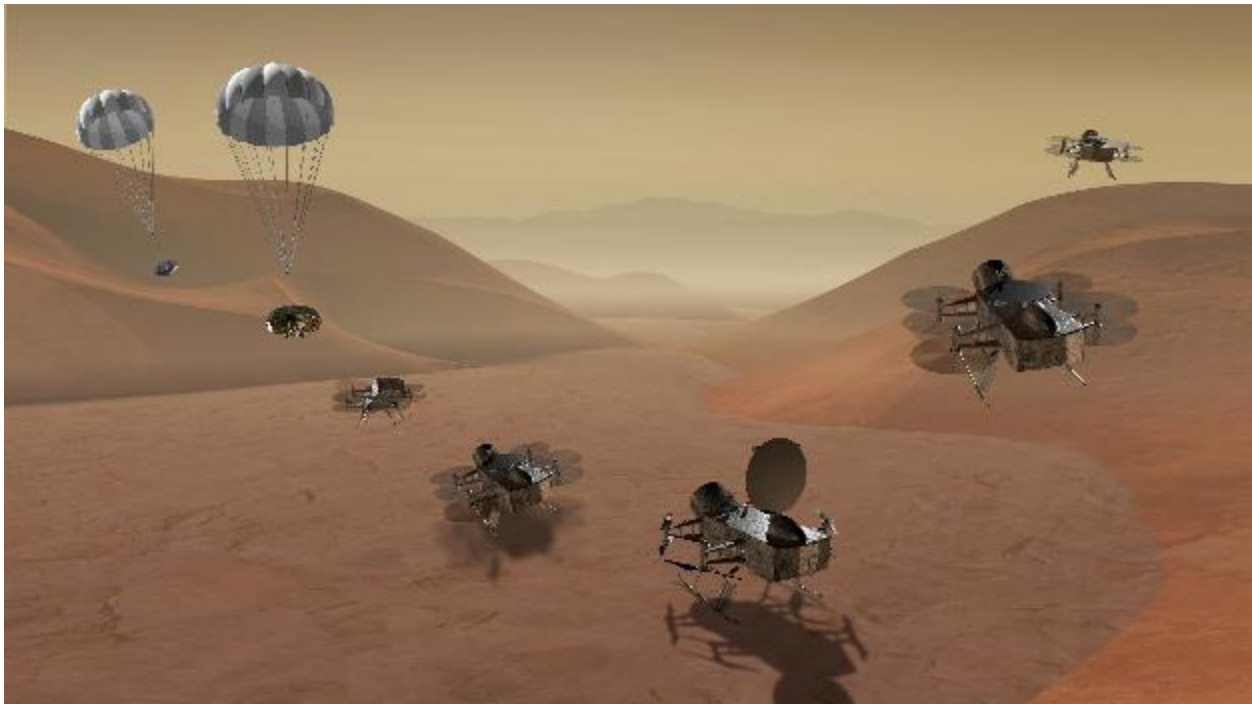
FIGURE 3.8 An artist's conception of Dragonfly, a rotorcraft lander is designed to explore Titan. It is currently under study as one of two possible candidates for NASA's fourth New Frontiers mission for launch in the mid-2020s. SOURCE: Courtesy of Johns Hopkins University Applied Physics Laboratory/Steve Gribben.
