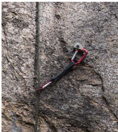
In rare cases, it’s possible for a carabiner gate to lever against a bolt and unclip. The top biner in this draw should be oriented in the same direction as the rope biner. Erik Rieger
