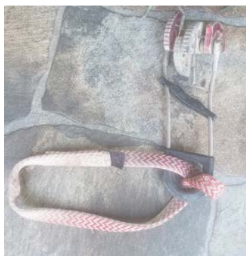
This vintage cam, found in a Zion crack, failed as a makeshift rappel anchor despite testing. Benton Mitchell
