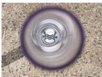
Looking down a turbidity tube. These tubes are useful for measuring suspended solids in runoff water.
