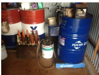
Store oils on an impervious surface, preferably with bunding.
