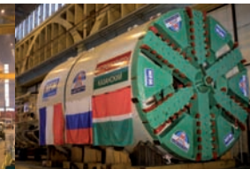
Soft ground TBM
