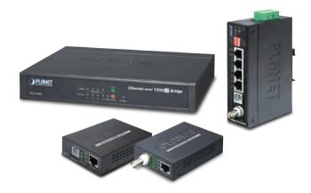
PLANET VC series is Ethernet-over-VDSL2 Media Converter with high performance. It is based on two core networking technologies, Ethernet and VDSL2 (Very-high data-rate Digital Subscriber Line 2). The VDSL2 technology offers the absolutely fastest data transmission speeds over the existing copper telephone lines without the need of rewiring.
